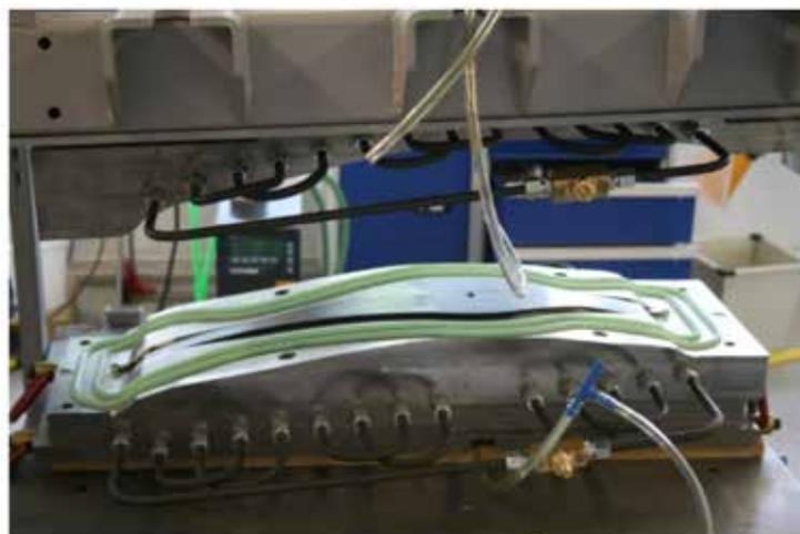
Figure 3: Separating the two mould halves after injection, exposing the semi-finished product. Note the tubing used for resin transport.
