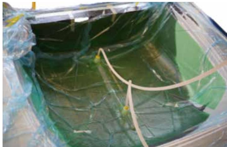
Figure 6: Vacuum infusion of a (part of a) ship's hull. The resin "front" is visible as the line between the dark and light green of the resin distribution medium.
